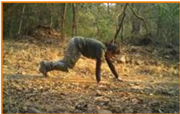
A test walk must be done at the level of the target animal, to test the proper functioning of the camera
